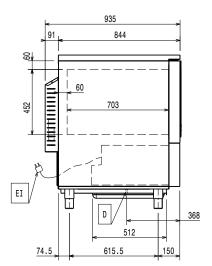
Drain Electrical inlet (power)
